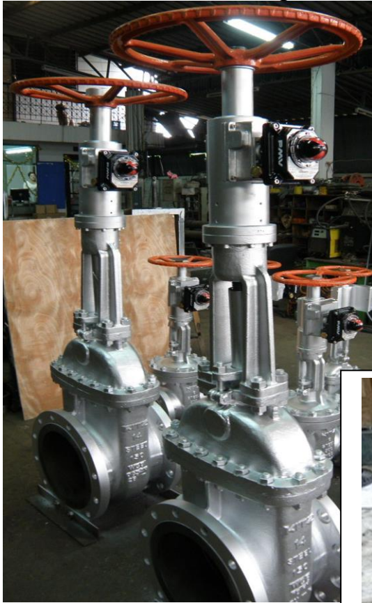
VSTNV-20 with FLOWSERVE switch box mounted on KITZ 12" gate valve
