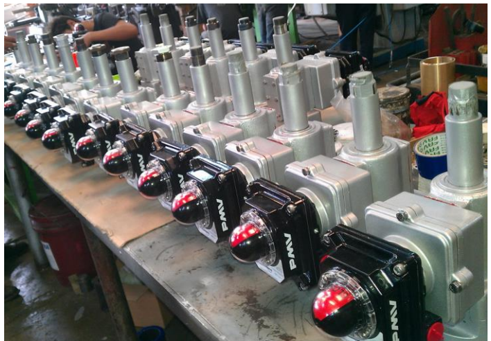
ValveSense Modules to be retrofitted to existing valves in ThaiOil 2013
