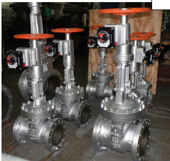
VSTNV-12 mounted Kitz valves Client : Thai Paraxylene Co., Ltd.
