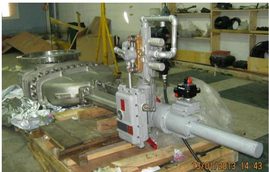
ValveSense Module as Auxiliary position feedback for EIM Pneumatic Multi-turn Actuator
